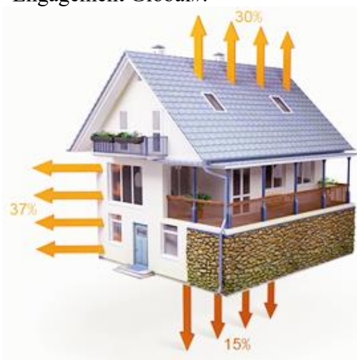
Fig. 1. Estimated heat loss in the building
